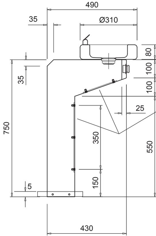
3mm S/S access panels fixed with M5 CSK security screws
