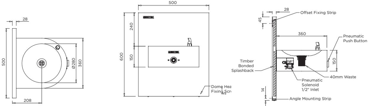
MODEL DDR1-C Plan, Front Elevation and Side Elevation
