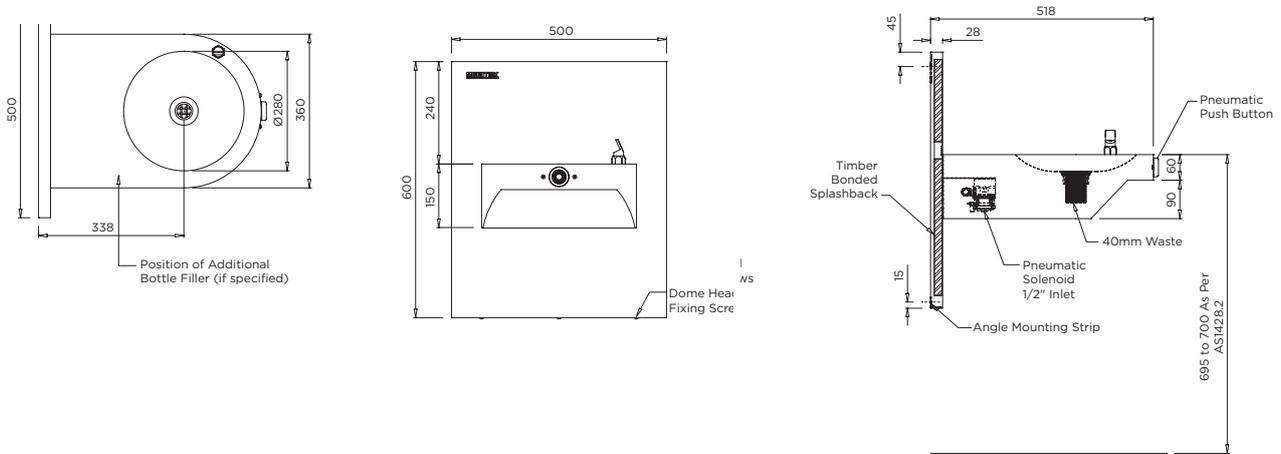
MODEL DDR1-D Plan, Front Elevation and Side Elevation
